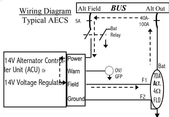
If there is voltage drop in the input devices preceding ACU, due to high resistance, the system will not work correctly. For example, this alternator with 4Ω field resistance draws 3A at 12V and 3.5A at 14V. *Ohm's law again.*
